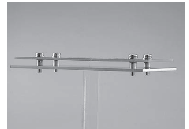
Condition of fitting the PC board to the chassis
