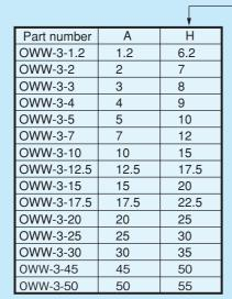
The dimension H indicates the distance between the main board and the slave board when PMW-61 is used.
